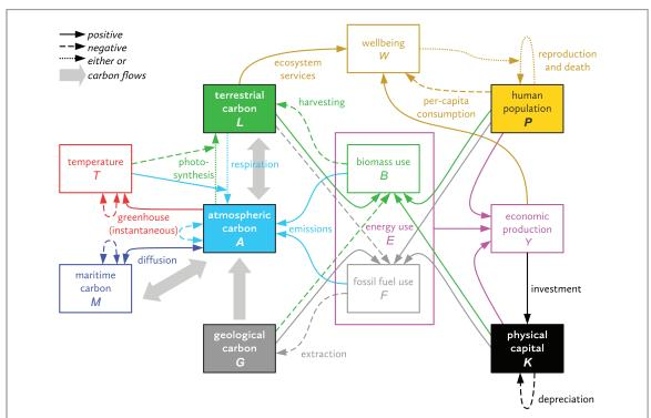
**Figure 1.** Overview of the model structure with five state variables (colored boxes) and several derived variables (white boxes). Arrows represent coupling processes between the variables. The left part represents the natural subsystem of the Earth (Ecosphere) via the global carbon cycle, while the right part represents socio-economic entities related to human activities in the World (Anthroposphere).
